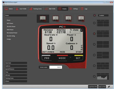
After downloading and installing the application, connect the PC8 to a USB port on the computer using the charging/download cable. Open the Device Agent software - a connection icon in the status bar will indicate that communication with the PC8 is established.
